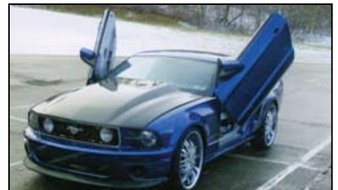
2007 Ford Mustang David Hazinski, Finletville, PA Vertical door hinges, Saleen Front bumper
